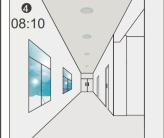
When the natural light level exceeds setpoint off to light will turn off even if when the space is occupied.
